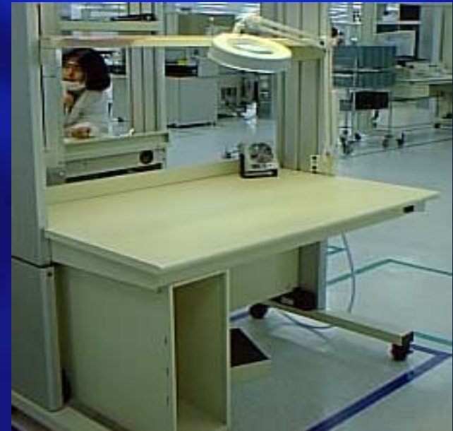
Typical ESD Workstation
